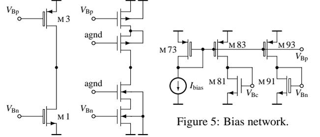
Figure 4: Cascode transistors.
