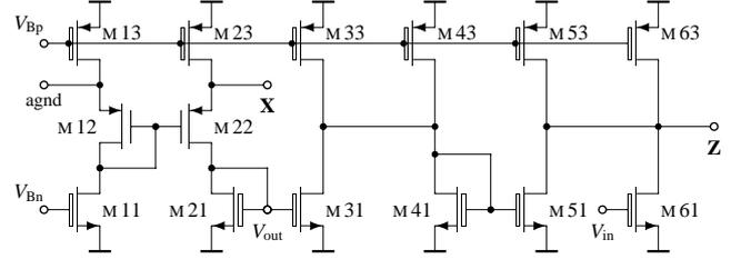
Figure 3: Current amplifier half-circuit.
