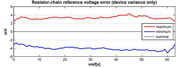
Fig. 5. Layout of the resistor chain with horizontal resistor elements and vertical metal lines to access them, including dummies (top) and worst-case errors on the different  $x_i$  obtained with 1000 Monte-Carlo runs (bottom).
