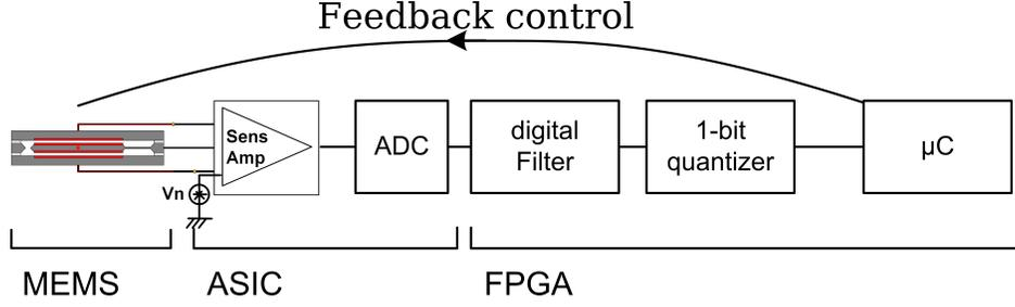
Fig. 1. Block diagram of a  $\Sigma\Delta$  accelerometer loop.
